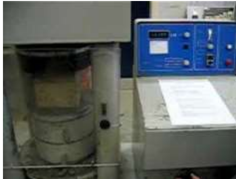
Figure 4 Concrete Cube Test
